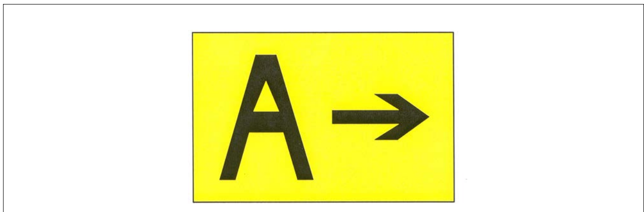
FIG 2-3-36 Direction Sign for Runway Exit
