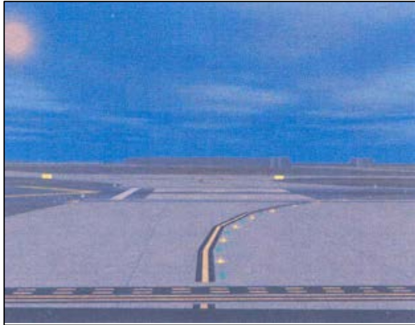
FIG 2-1-12 Taxiway Lead-On Light Configuration
