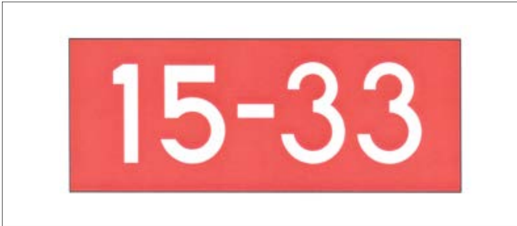
FIG 2-3-24 Runway Holding Position Sign
