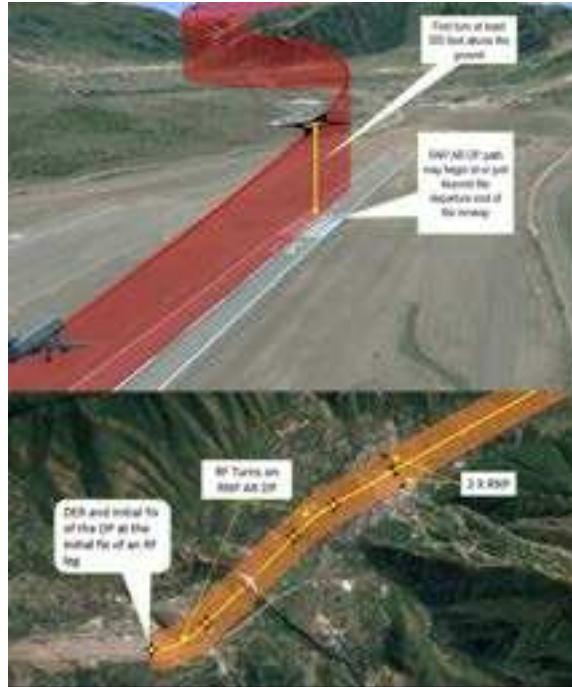
FIG 5-4-26 Example of an RNP AR DP
