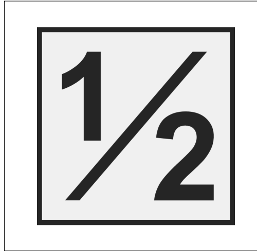
FIG 7-6-1 Typical Runway Half-way Sign
