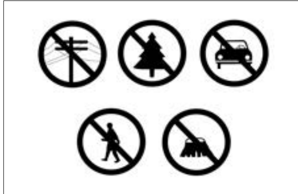
FIG 10-2-5 Landing Zone Hazards
